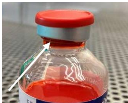
Fig 1. Example of vial closure abnormality
